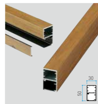
Louver Furring strip Size in mm 30x50xL4000 t:1.2mm
