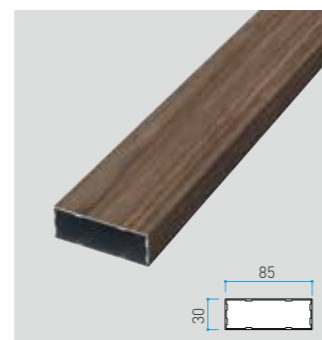
Louver 85x30 Size in mm 85x30xL4000 t:1.0mm
